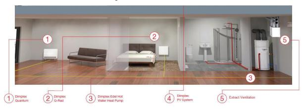
Figure 6: Typical Air-Source Heat Pump with Electric Panel Heaters Arrangement
