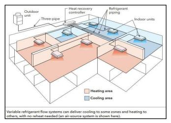
Figure 9: Typical VRF Schematic Diagram
